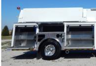
Spartan FC-94 MFD 10" Raised Roof Chassis Cummins L9 450 HP Diesel Engine Allison 3000 EVS Automatic Transmission Heavy Duty Aluminum Body and Sub-Frame Four (4) Person Cab
