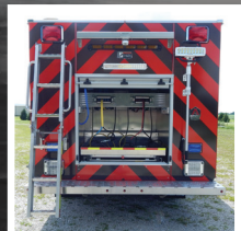
Dual Hydraulic Reels, Customized Tool Mounting
