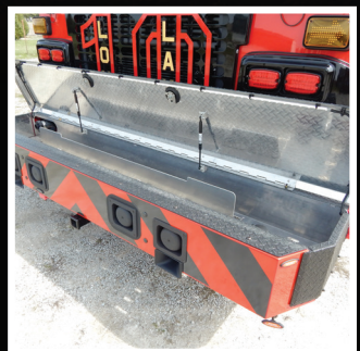
Customized Front Bumper Storage Compartment in Various Configurations for Different Functions
