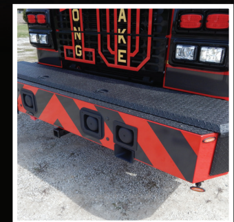
Customized Front Bumper Storage Compartment in Various Configurations for Different Functions
