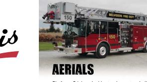
Platform, Stick, or Ladder trucks custom built with a variety of ladder sizes and types, Smart Truck Logic based controls, wireless remote controls, breathing air, a retractable waterway, operator's chair and joystick controller, and tip-mounted equipment. Choose from top-of-the-line lighting and accessories and fully customizable storage compartments.
