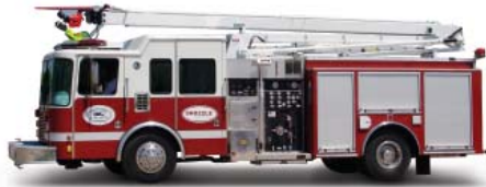
AERIAL SNOZZLE DEMO 65' Snozzle with tilt 15' below grade and light weight, multiple position water tower.
