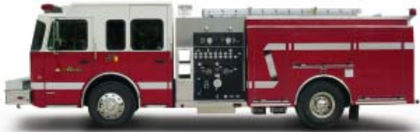
PUMPER DEMO 1894 Custom Side Control Pumper with a Spartan Flat Floor Advantage MFD and 10" raised roof.
