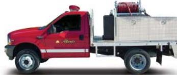
BRUSH TRUCK DEMO SK666 Flatbed Mini with heavy-duty aluminum body and Waterous 18hp Gasoline Pump for grassland applications.
