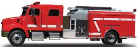
PUMPER DEMO 1903 Crew Cab Top Mount Pumper with a heavy duty 3/16" aluminum body.
