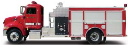
PUMPER DEMO 1902 Top Mount Pumper with Peterbilt Model 330 Chassis and 1000 gallon UPF Poly Tank IIE.
