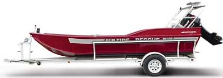
CYCLONE 1760V DEMO U.S. Coast Guard approved 17' heavy-duty rescue boat with marine aluminum alloy constructed sides and bottom.
