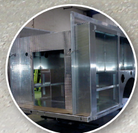
All-welded 3/16" aluminum body
