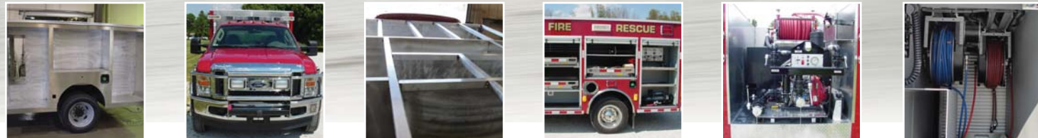
All Welded 3/16" Aluminum Body Top-brand lighting and accessories Structurally Supported Roof Customized Storage Compartments Slide-In Skid Units Available Dual Hydraulic Hose Reels, Transverse Compartment
