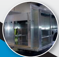
All-welded 3/16" aluminum body
